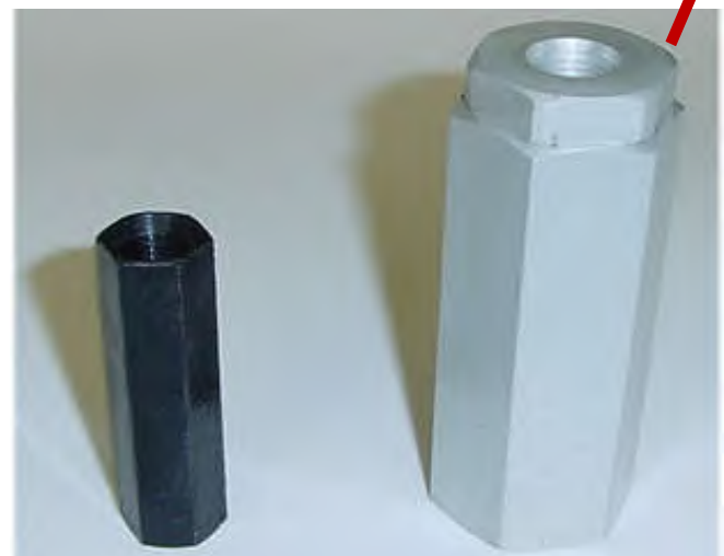
Photo showing the difference in size between part no. A110079 (left) and A249366 (right).
