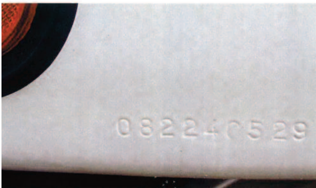
Nine Digit Serial Number Stamped Into Frame
