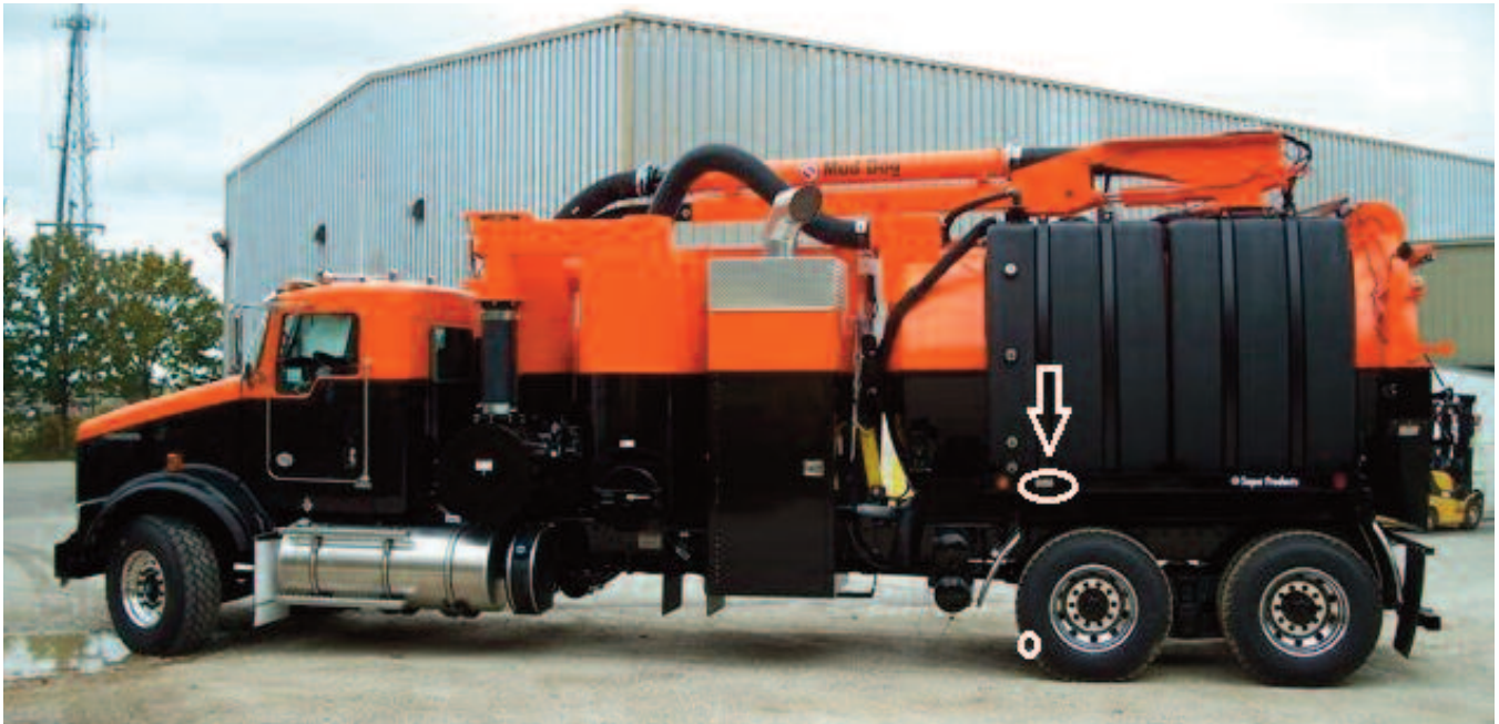
Locating Serial Number on Super Products Mud Dog - 2001 to Current
