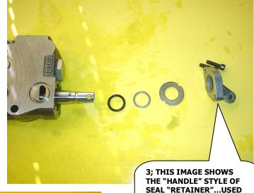
THE "HANDLE" STYLE OF SEAL "RETAINER"...USED AT LEGACY3'S <u>"BODY</u> MOUNTED VALVE"...REUSE THIS WHEN REPAIRING THE "SEAL" HERE
