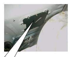
A "TYPICAL" CHASSIS PTO "ACCESS" HOLE IN THE CAB'S FLOOR...HELPFUL FOR PTO/PUMP "WORK" SEC 07-- PG 16 LEGACY 3
