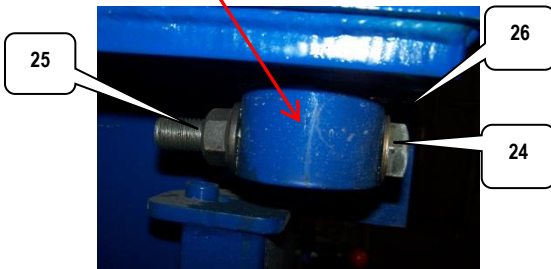
Left Side Packer – Cylinder Pins – Assembly
