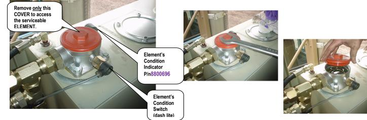
2- Remove the Filter's Top Cover by turning CCW. The Cover's compression spring will be "pushing"...so use your hand over the Red removable polymer cover when it is close to being fully un-threaded to control.
