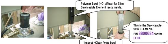
4- Now remove the "old" element. Put it into clean garbage bag so you can later "study" what has been trapped-out of the hydraulic system (can offer "clues" as to the hydraulic system's "health").
