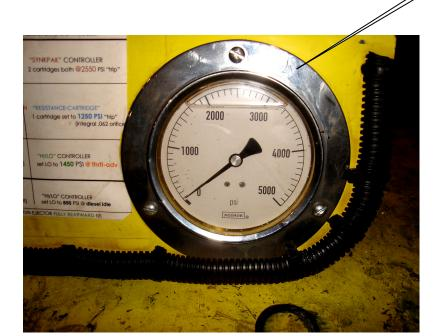
Every LOADMASTER Body will have a **Male Gauge Stem** at the Inlet Cover of "Body-Mtd Valve"...this is PUMP PRESSRE...**ALL** LOADMASTER "pressure checks" are done **at** <u>this</u> Gauge Point.
