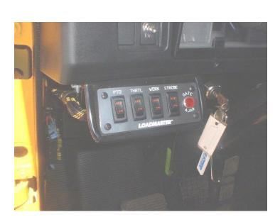
Turn on your beacon or strobe lights (and the hopper area work lights, if needed) by positioning the rocker switches so that the red band is exposed.
