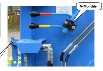
**U)** Left/Right Cart Tipper Hand Valve Lever Pivot (if equip'd) V) Bearing Blocks for Blades Levers (Lower & Upper)
