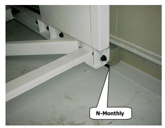
Left/ Right: N) Ejector's Body Tracking Channels/Shoeings
