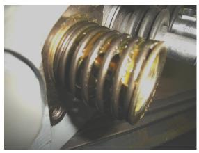
NOTE: Assure the correct "Orientation" of items 1 & 2 as imaged here (Assure CORRECT orientation...or seal system will "fail")
